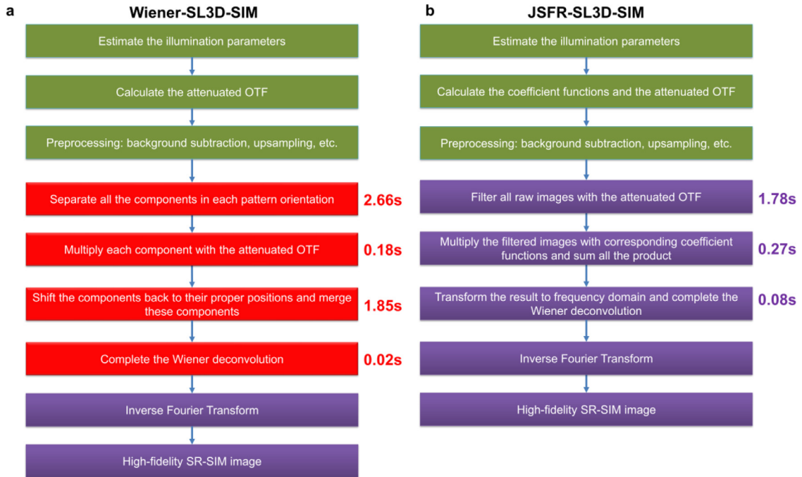
Fig. 2. Comparison of the computing burden of the conventional Wiener-SL3D-SIM (a) and the developed JSFR-SL3D-SIM (b). To provide an intuitionistic impression of the source of computing burden, the execution time of each main procedure in the two algorithms is listed on the right-hand side of the diagrams, which was tested in CPU (Intel Core i7-9700 K) with a raw image size of 1024 \times 1024 .
